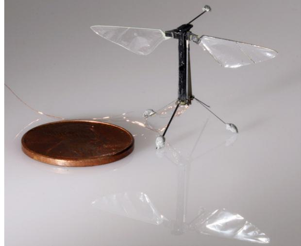
Fig. 1. Photograph of one of the flapping-wing flying microrobots used in the work presented in this paper. The prototypes considered in this work have two completely independent lateral actuators used simultaneously for power and control. The ball-shaped markers glued to the robot are used by a Vicon motion capture system in the estimation of position and orientation of the robot. This robotic prototype was entirely developed and fabricated at the Harvard Microrobotics Laboratory.
