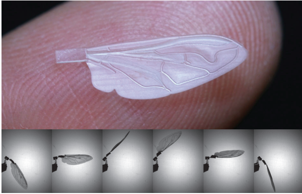
Fig. 6. Photo of a micromolded polymer wing mimicking the features of an Eristalis wing (top). This wing was created in a single molding step and includes veins ranging from 50–125 \mu\text{m} thick, 100 \mu\text{m} corrugation, and a 10–20 \mu\text{m} membrane. A sample of the wing motion (dorsal perspective) at 150 Hz flapping frequency taken from a high-speed video (bottom).
